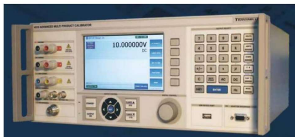
Figure 3. LEM reference standard multifunctional calibrator Transmille 4015 with inductance calibration option
