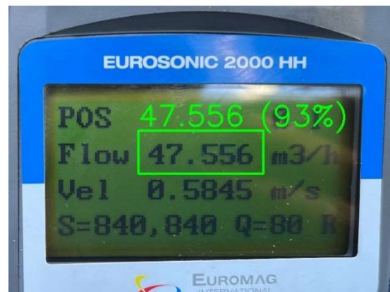
Figure 19: OCR result and confidence overlaid in the numerical display image
