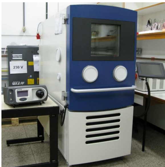
Figure 1: Dew-point hygrometer and the climatic chamber used in the experiments.
