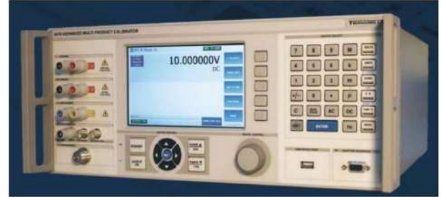
Figure 7. LEM reference standard multifunctional calibrator Transmille 4015 with oscilloscope calibration option SPC600
