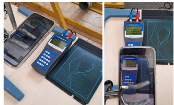
Figure 16: Close up of the flowmeter's numerical display and the smartphone for image streaming
