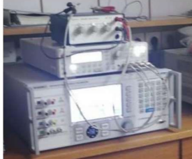
Figure 6. Test set-up in LEM for calibration of ROHDE & SCHWARZ HM8118 LCR-Bridge with the Transmille 4015 Multifunctional Calibrator
